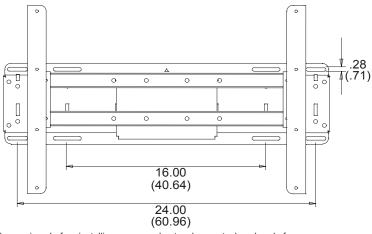
Note: Measure Back Plate demensions before installing power and network receptacles ahead of of installation to avoid conflicts.
