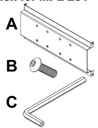
Mount display adapter to back of display unit securly. Adjust sliding adapter screws to fit TTUFF PC unit. Place TTUFF Mounting bracket (A) onto plasma adapter, then align all holes and attach mounting adapter using four screws
